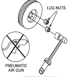
TORQUE WRENCH Figure 57. Wheel Lug Nuts Tightening Sequence
